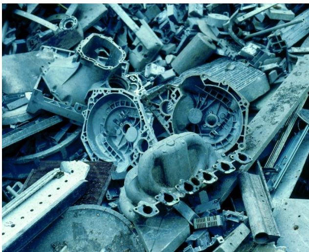
Figure 1.0 Aluminium scrap from ELVs; source: Kirchner VAR Verband der Aluminiumrecycling-Industrie e.V.
