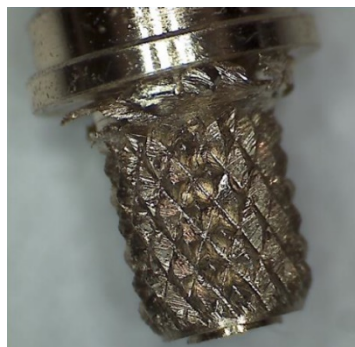
Figure 21. A knurl made from CuZn42 with sharp edges and broken material.
